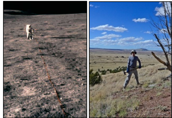
Figure 1. Left: Apollo 14 astronaut Edgar Mitchell operates the Thumper for the Active Seismic Experiment. Right: Astronaut Don Pettit prepares for an active source seismic shot in the SFVF that replicates the geometry of the lunar experiment. Image Credits. NASA, J. Richardson
