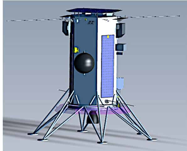
The figure above shows the NOVA-C lander with several payloads, including our four deployed Stacer antennas. Two are mounted at ~1 m above the lunar surface; the other two are mounted at ~3 m above the lunar surface. Their front-end electronics units are all connected to the Main Electronics Box, which is not shown.
