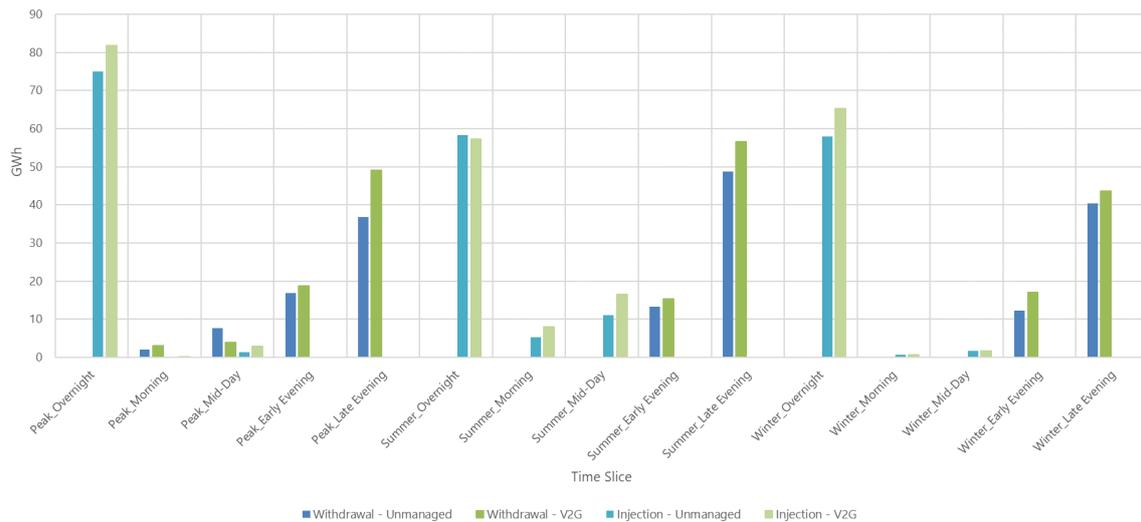
Figure 14: Withdrawal from and injection into total storage capacity for the Net Zero Unmanaged Charging and V2G scenarios in 2050
