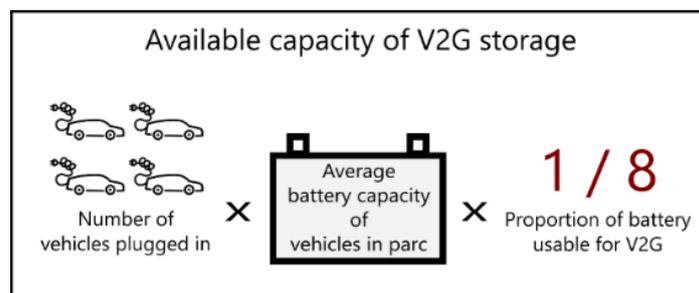
Figure 2: Calculating the aggregate V2G capacity available
