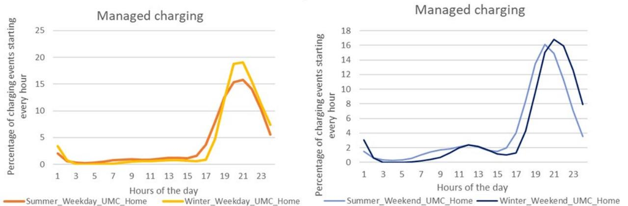
Figure 6: Hourly charging demand of BEVs for User-Managed Charging (UMC) scenario on weekdays (left) and weekends (right)
