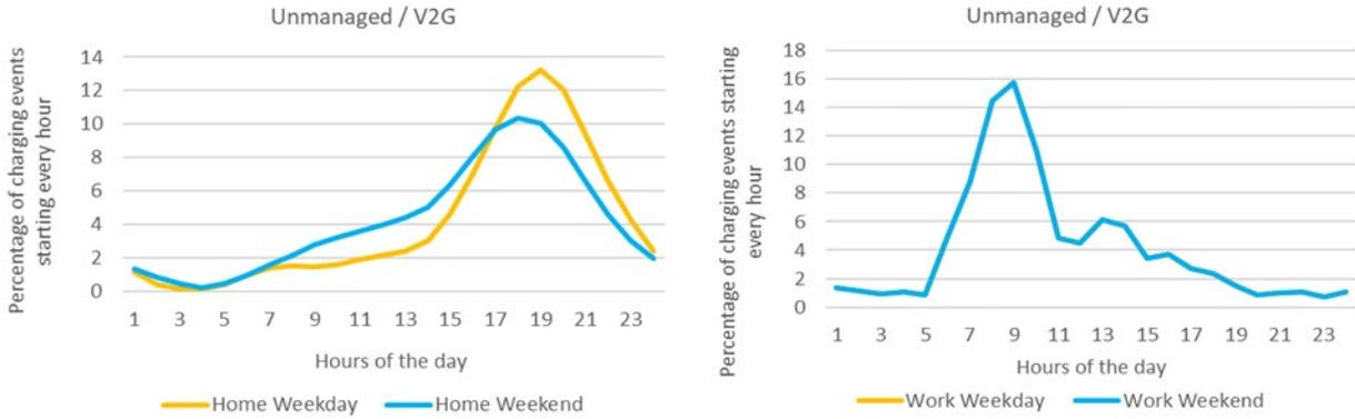
Figure 5: Hourly charging demand of BEVs for unmanaged charging and/or V2G scenarios at home (left) and at work (right). Due to a lack of data regarding weekends, charging profiles at work are the same on weekdays and weekends; a weighted average is used to combine both into a single typical day
