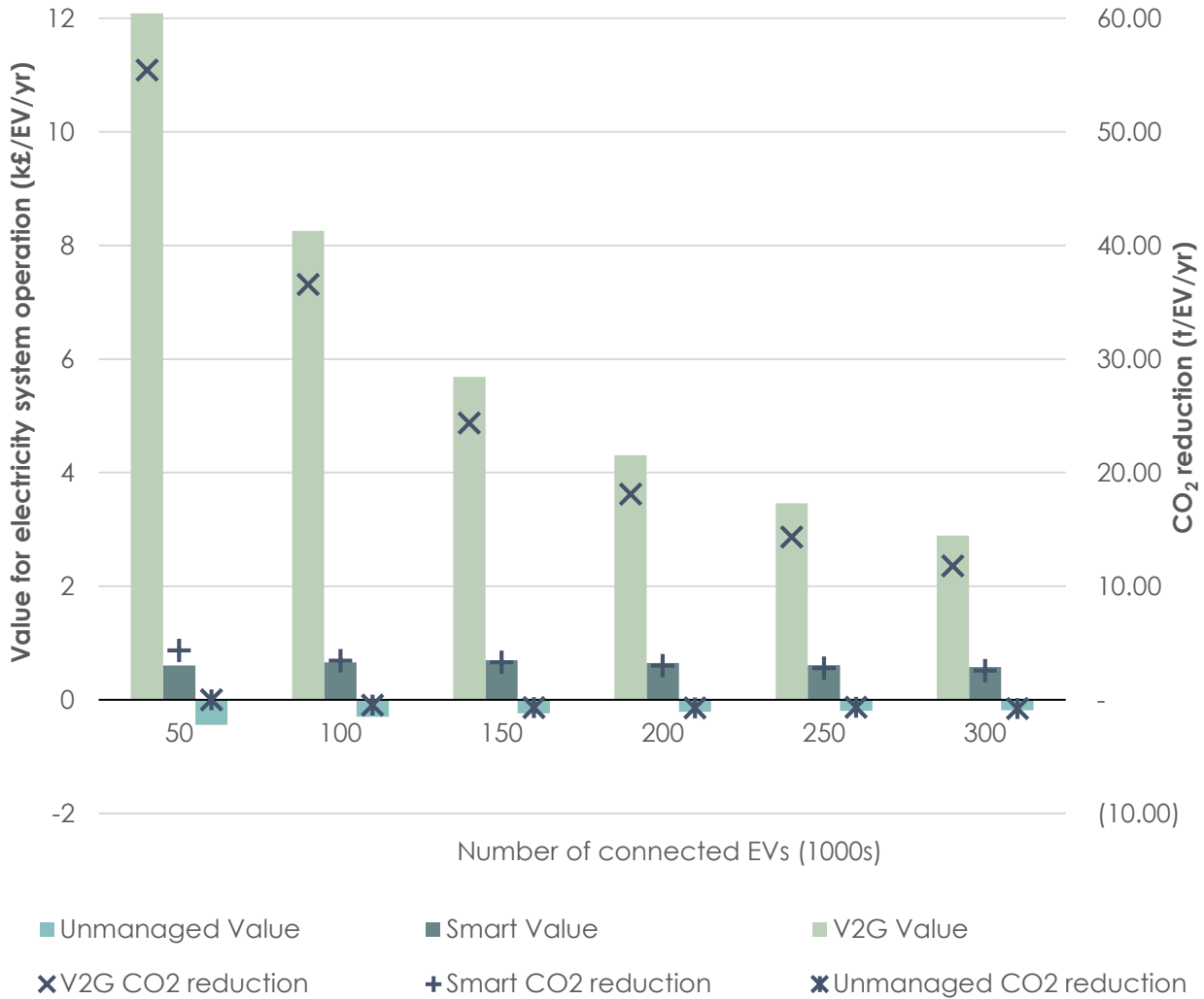
Figure 8: Annual net operating cost savings and CO2 emission reduction per EV for various charging regimes and EV penetrations
