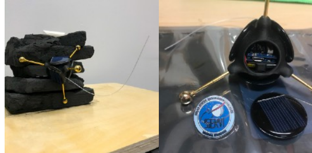
Figure 1, Left: The fully-functional 48-gram seismic sensor mote, magnetically anchored to an irregular vertical wall of Phobos regolith simulant. Caltrop shape enables three of four legs to contact surface in spite of irregularity. Whip antenna also shown. Right: Interior of the seismic sensor mote, showing the tightly-packed electronics, which include the C&DH computer, battery and PMU, instrument, and radio transceiver. SSERVI pin is 25 mm in diameter.
