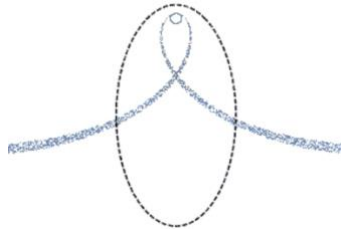
Figure 1. Cross sectional view of lunar lander ejecta (blue dots) leaving the Moon (small circle) from the landing site (top of the circle). Ejecta cross the Lunar Gateway orbit (dashed ellipse).
