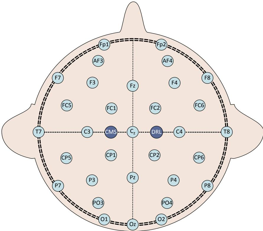
**Fig. 4.2** An example of the 10–20 electrode placement
