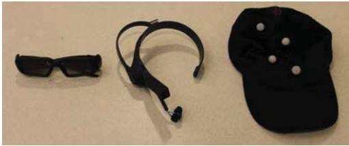
Fig. 3. Apparatus used: NVIDIA active shutter 3D Vision Pro glasses, Neurosky Mindwave Mobile, and IR tracking capable cap.
