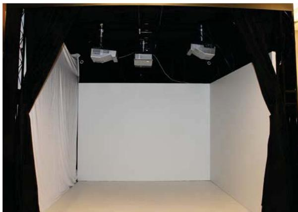
Fig. 1. Four-wall CAVE (2m x 2m), Panasonic projectors (1024x768 resolution), and Vicon IR tracking system at UOIT.
