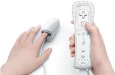
**Figure 2.** Prototype of the planned Nintendo Wii Vitality sensor, a pulse oximeter.
